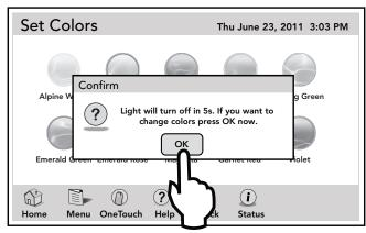
NOTE When a pool or spa light is turned ON manually, by the OneTouch™ control panel, or by a program, the last used color will automatically be chosen unless you press SELECT to change the color.
