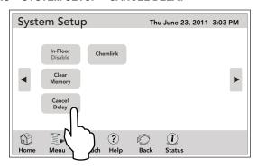
CANCEL DELAY should only be used by authorized service personnel. It should not be used during normal system operation.
