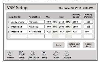
In the PUMP MODEL list, select the variable speed pump type and click the SELECT button to save it.
