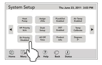
When solar and heater are enabled the solar will heat the water until either the thermostat setting has been reached or solar heat is no longer available. If the solar panel is not hot enough, solar heat will shut off and the other heat source (usually gas heater) will take over to bring the water up to the thermostat setting. This menu is used to ENABLE or DISABLE the solar priority.
