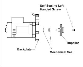
Figure 5. Remove the Impeller
