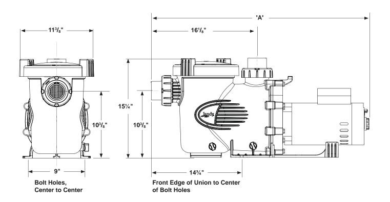
**NOTE** When installing pump, leave a minimum of two feet (2 ft) of clearance above the pump for removal of strainer basket.
