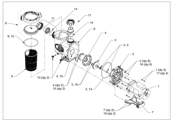
Figure 10. SHPF and SHPM Exploded View
