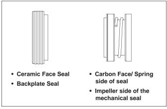
Figure 8. Replace the Mechanical Seal
