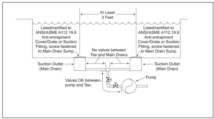
Figure 1. Number of Suction Outlets Per Pump
