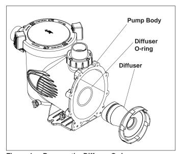
Figure 4. Remove the Diffuser O-ring
