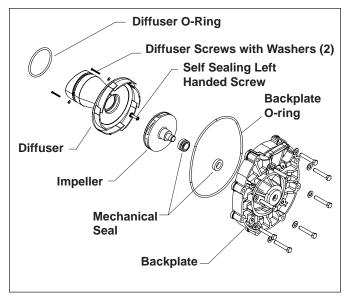
Figure 6. Diffuser and Impeller Exploded View
