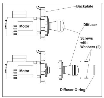
Figure 3. Remove the Diffuser
